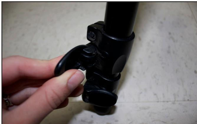
Open the latches on tripod legs, extend each to desired height and lock.
