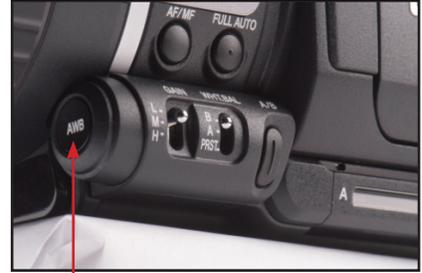
**White balance** camera by zooming camera into a white piece of paper/object and pressing AWB (tip: set up lighting and shot before WB so that the same light is captured on camera)
