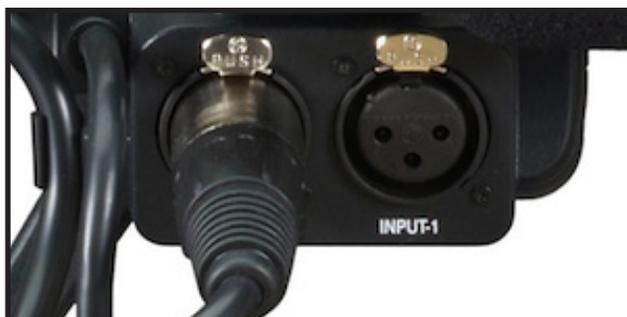
Inputs for external audio devices. Make certain that the inputs are on the correct channels.
